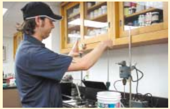
A viscosity test is performed on an ink sample.
